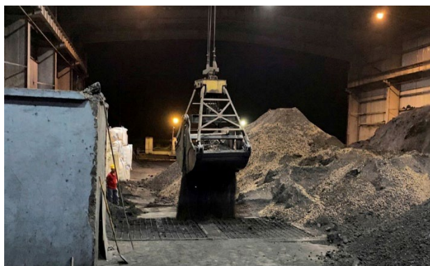
Feeding of the Wood Pellet-Coal Mixture
