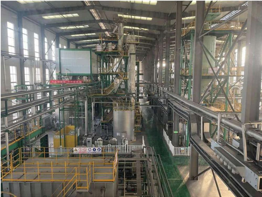
The "Lithium Ion Battery (LIB) Recycle System" is a system that recovers rare metals from used automotive LIBs with high efficiency and low environmental impact. The rare metals contained in automotive LIBs are recycled, and highly efficient lithium recovery is made possible by improving energy efficiency, such as by using exhaust gas from cement manufacturing facilities from the preliminary roasting to roasting process.
