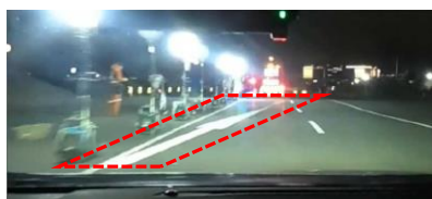
LED projector evaluation Lane guidance display projected by arrows in red frame
