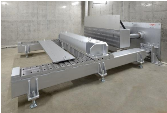
Crush Testing Equipment (No. 1 Safety Test Room)
