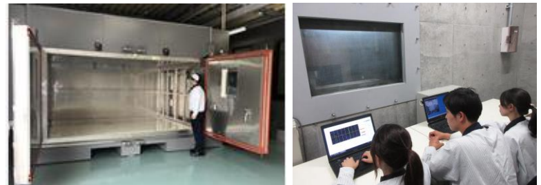
Capable of performing various safety tests for secondary batteries compliant with United Nations regulations and other standards Battery Safety Testing Center
