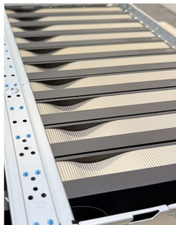
New server system with 10 NVIDIA RTX 6000 Ada high-end GPUs
