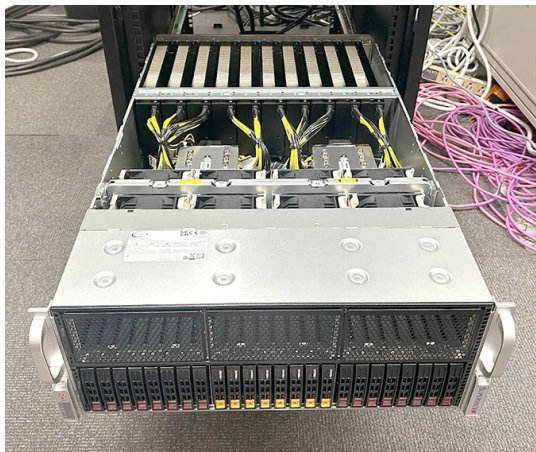
New server system with 10 NVIDIA RTX 6000 Ada high-end GPUs
