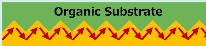
Surface roughness approximately 2um (Skin depth approximately 0.4um @28Ghz)
