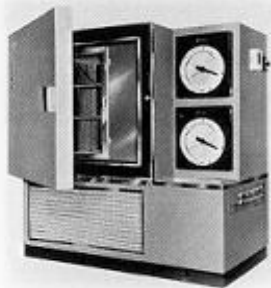
Low Temperature & Humidity Chamber "Lucifer"
