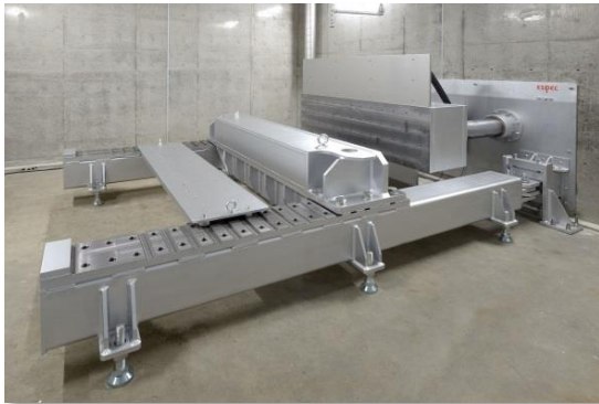
Crush Testing Equipment (No. 1 Safety Test Room)
