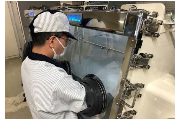
Glovebox for dismantling cells
