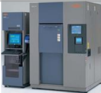
Conductor Resistance Evaluation System
