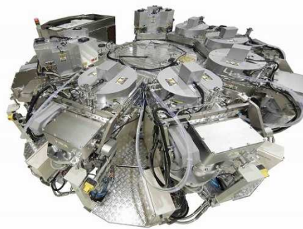
8 chamber configuration (7 process chamber and load lock)
